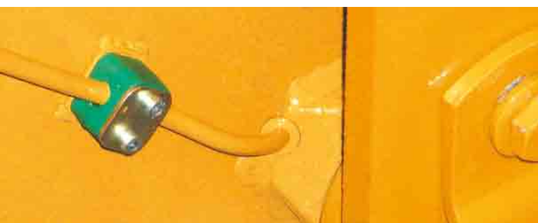
Bearing insert adaptor for 10mm thick tube
